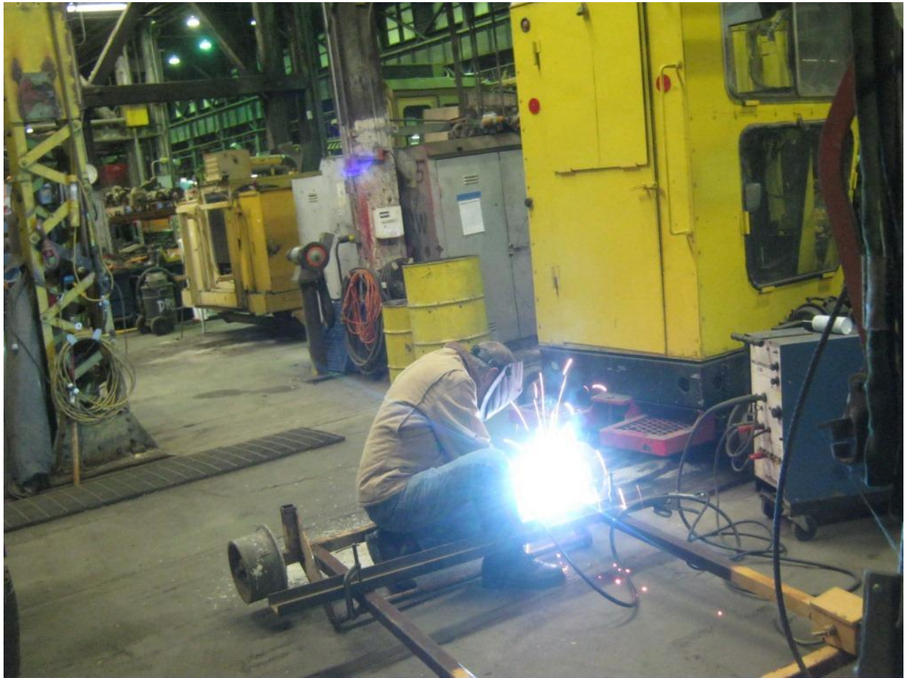
Alan welding the surfacing system for the “new-old” tamper together
