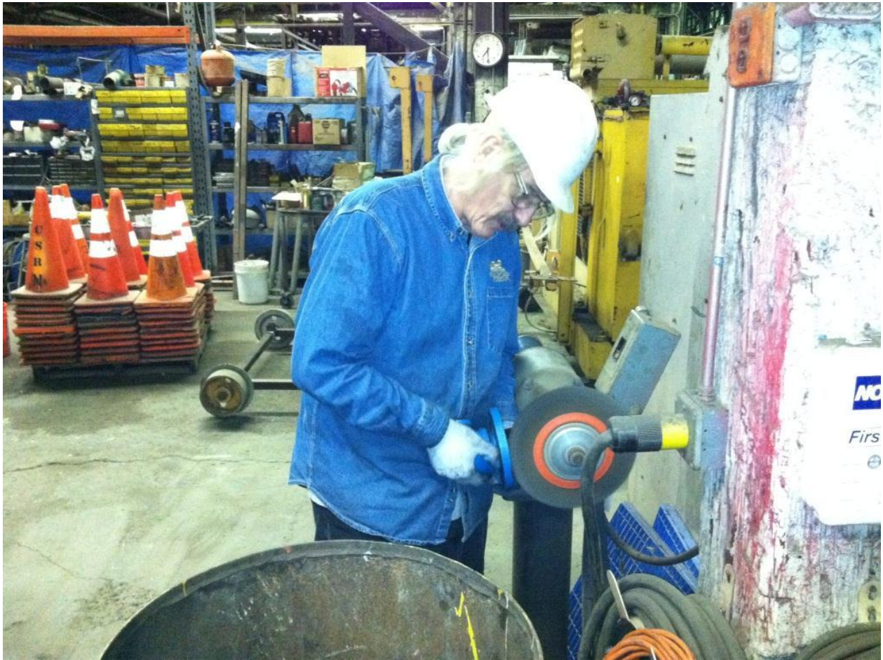
Fred using the wire-wheel on a component of the hydraulic tank
